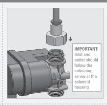
The faucet is provided with an inlet nipple. If needed, fit the water supply inlet to the inlet nipple at the solenoid valve housing in the dual power input box or connect it directly to the shut off valve.
