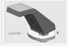
For Condor \ Condor E only: slide the disk, washer and nut over the faucet left and right studs and secure them.
