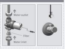
Note: Make sure that the filter is assembled between the housing of the solenoid valve and the adapter.
