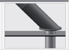
Slide the gasket, disk and hexagonal nut over the flexible hose and secure the faucet into place.
