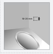
Insert the faucet base through the wall and fix it firmly on the opposite side with the hexagonal nut and the disk.
